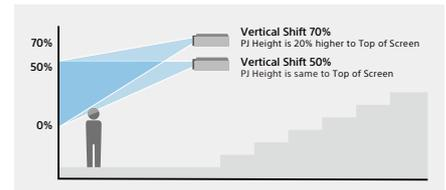
The projector has variety of lens options and wide lens shift capability for flexible installation, virtually anywhere.
