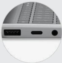
Built-in USB-C®, USB-A and Surface Connect ports, headphone jack
